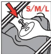
Just unscrew the sizing screw and the big yoke bolt, slide the runners to the desired position, then reattach both.
